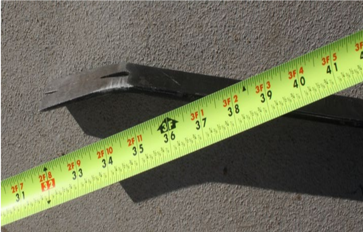
Photo 4. The pry bar the installer was using with a tape measure showing the distance the pry bar was found from him after he fell.
